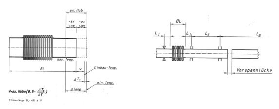
As a matter of principle, when installing all expansion joints, care must be taken to ensure that the expansion joints are not affected by unfavourable pipe movements, for example as torsion.
