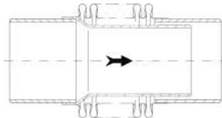
Intended Insulation in the area of the expansion joint must be agreed with Flexomat GmbH.
