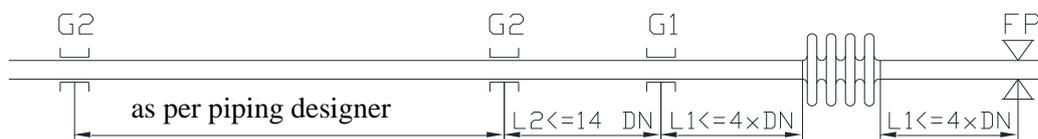
G1 and G2 => Friction bearing    FP => Fixed bearing
